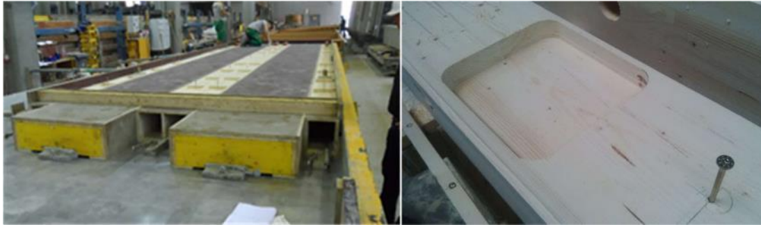
Figure 3.7 Hybrid Slab in production (Image Copyright: CREE GmbH, www.creebuildings.com )
