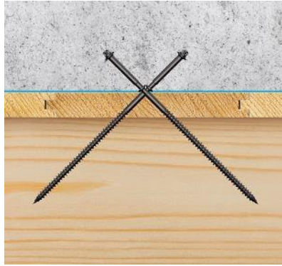
Figure 2.4 Specialised SFS VB screw for TCC (DiBt 2018; SFS intec 2016)
